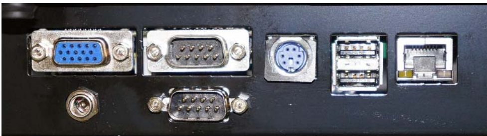
VGA out Screw-type DC power 2-Serial PS2 2-USB Gigabit Ethernet
